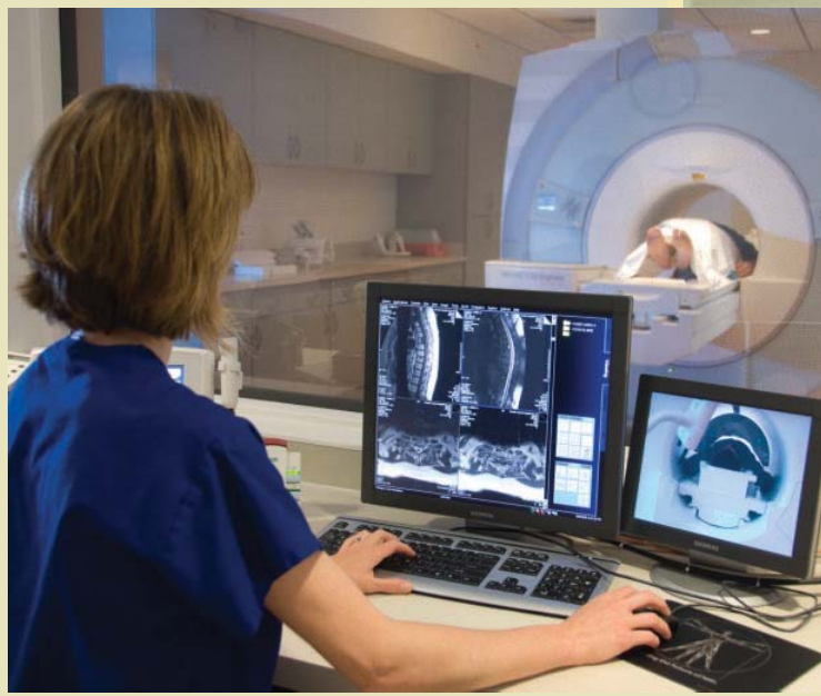
Melinda Ryan, MRI Technician, operates the Siemens Espree, which is a 1.5 high field, short bore, semi-open unit
